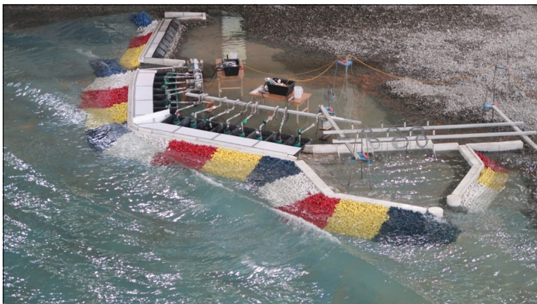
Photo 1. Photograph of hydraulic experiment showing the sea wall and the overtopping measurement devices.
